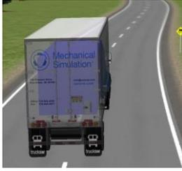
Fig. 9. Animation with a 312 state model in TruckSim
