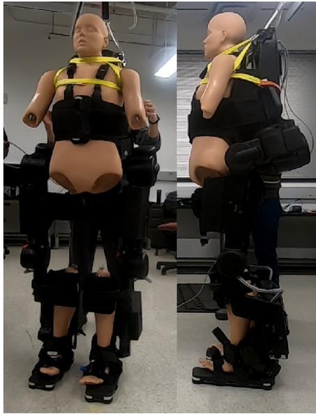
Fig. 7. Setting of exoskeleton ATALANTE with a mannequin.
